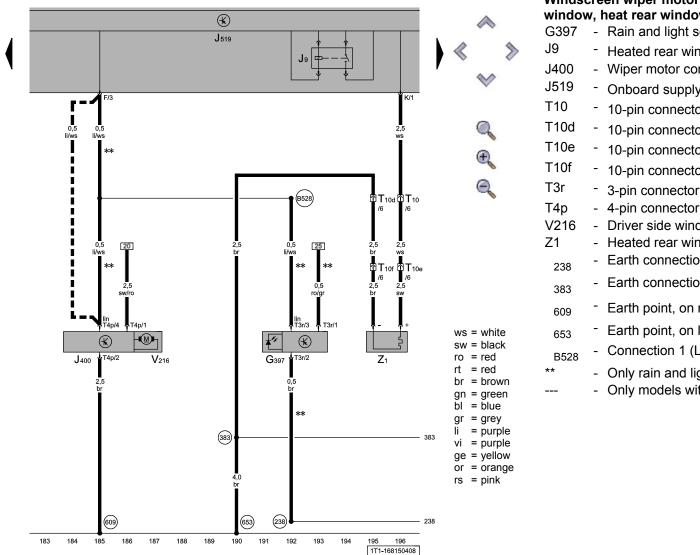
Windscreen wiper motor on driver side, relay for heater rear window, heat rear window, sensor for rain and light detection
