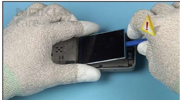
18. Very carefully lift the LCD from the MAIN FRAME.
