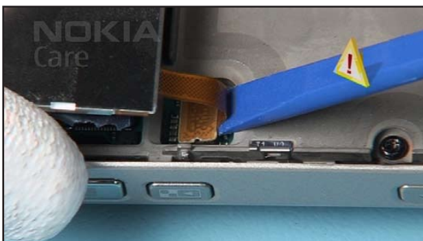
19. Gently open the LCD connector.
