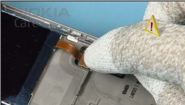
33. Close the LCD connector.
